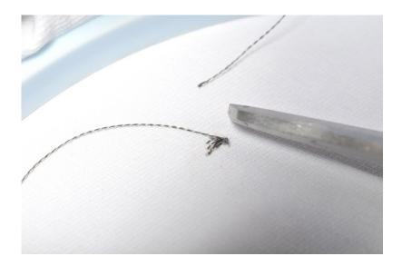
When dry, trim the tail end of the thread very closely to the sealed knot. Now you can continue stitching with the long tail to connect up different parts of your circuit!
