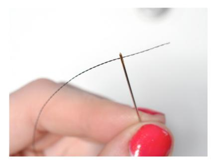
Thread a medium size needle with the conductive thread. You may need to moisten the thread end to help it stay pointy for threading.
