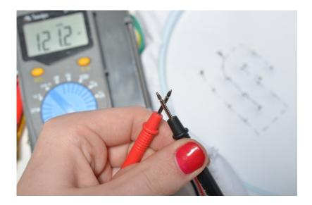
Use a multimeter's continuity tester to check your circuit for shorts. The meter will beep any time the two probes are electrically connected.
