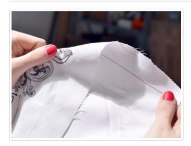
Leave long tails of conductive thread at the ends of your stitching lines in case you need to pick them up with a hand sewing needle and connect to other components.
