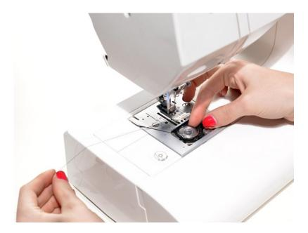
You can use our 2 ply conductive thread in the bobbin of a sewing machine. Thread the machine's needle with plain thread.
