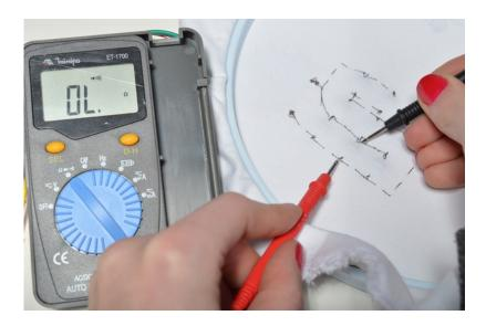
Put one probe on power and one probe on ground. There should be no beep!
