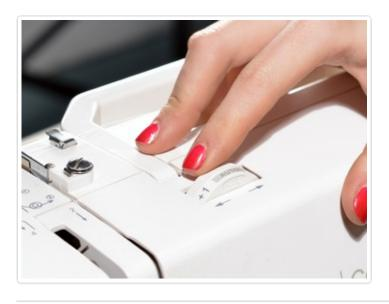
You may need to adjust the tension on your machine. Experiment on a scrap piece of fabric and examine the balance between the conductive and regular thread. Adjust the tension and experiment again until you are satisfied.
