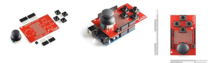
**Description:** The Joystick Shield kit contains all the parts you need to enable your Arduino with a joystick! The shield sits on top of your Arduino and turns it into a simple controller. Five momentary push buttons (4+ joystick select button) and a two-axis thumb joystick gives your Arduino functionality on the level of old <u>Nintendo controllers</u>. Soldering is required, but it's relatively easy and requires minimal tools. We even have a <u>step by step guide</u>!
