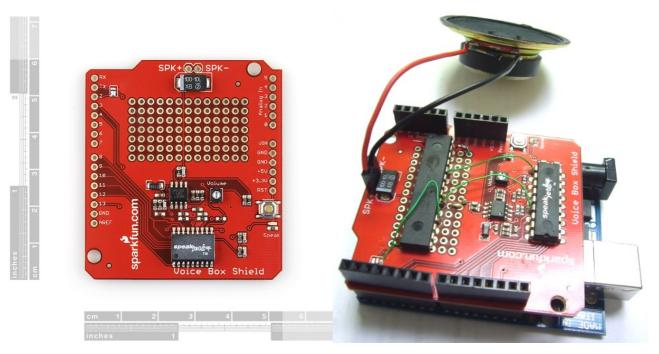
**Description:** The VoiceBox Shield can be mounted on top of your <u>Arduino USB Board</u> or <u>Pro</u>, to give it access to all capabilities of the <u>SpeakJet</u> voice and sound synthesizer. The Voice Box Shield uses the SpeakJet chip to convert serial commands into a great robot-sounding voice.
