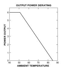
Typical Performance: (Tc=25°C, Vin=Nom VDC, Rated Load)
