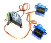
This is probably the smallest Arduino controller speically designed for controlling servos. It features a 12 standard servo control capbility with an Xbee socket which can be used in model helicopters or UAVs via the Xbee link. The feather weight (7.5g) makes it an ideal controller for application with a limited payload. The built in regulator allows the input voltage to vary from 3.5-8V which fits most power supplies without any modification.
