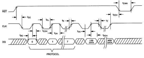
NOTE: t<sub>CL</sub>, t<sub>CH</sub>, t<sub>R</sub>, and t<sub>F</sub> apply to both read and write data transfer.
