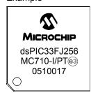
100-Lead TQFP (14x14x1mm)
