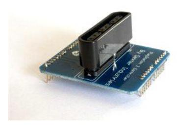
A Playstation DualShock controller interface for the Arduino. Slide this shield over your Arduino, plug in your controller, and you've got the awesome combination of a form-
