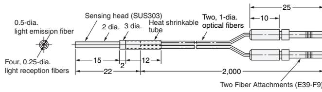
**Note:** The fiber for the emitter is identified by a white line.
