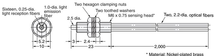
**Note:** The fiber for the emitter is identified by a white line.
