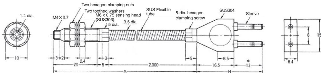
**Note:** Section A resists 300°C and section B (which is inserted to the Amplifier) resists 110°C. The operating temperature of the section to be inserted (marked with \*) must be within the operating temperature range of the Amplifier.
