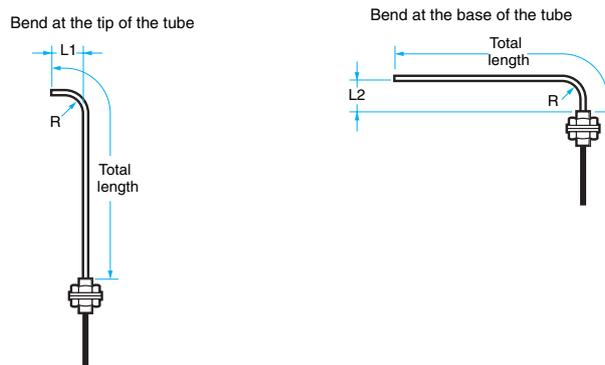
● **Model Numbers Incorporating the Bending Radius, R, and Dimensions L1 and L2**
