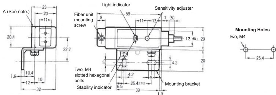
Note: The Mounting Bracket can also be used on side A.
