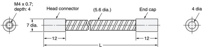
**Note:** The length L is 1,000 for the E39-F32C and 500 for the E39-F32C5.
