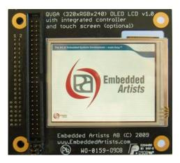
Embedded Artists' **2.8 inch QVGA OLED Display** *with touch screen* lets you explore the new Organic Light Emitting Diode (OLED) technology. OLED displays have better viewing angle, contrast, and brightness than LCD displays.
