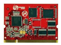
Embedded Artists' **LPC3152 OEM Board** is equipped with NXP's **ARM926EJ-S** based LPC3152 microcontroller suitable for a wide range of applications requiring low power consumption, high performance and flexible USB connectivity.
