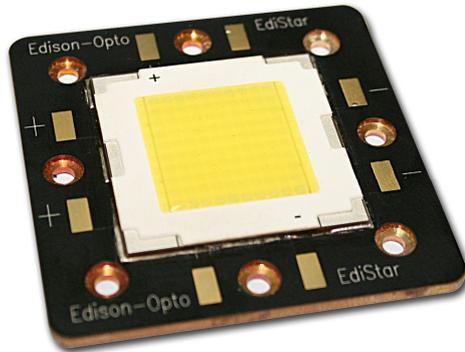
EdiStar series is the brightest LEDs in the world by Edison Opto. EdiStar series emitters are designed to satisfy more and more Solid-State lighting High Power LED applications for brilliant world such as general lighting, street light and projector light engine. EdiStar series emitters are designed by particular package for High Power LED. 50W and 100W EdiStar
