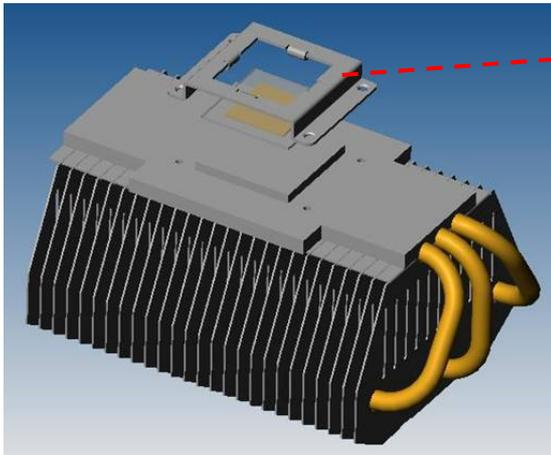
The function of cover (clip) is used to fix and force Edistar and heatsink to prevent the small gaps generate between the bottom surface of Edistar and the top surface of heat sink.
