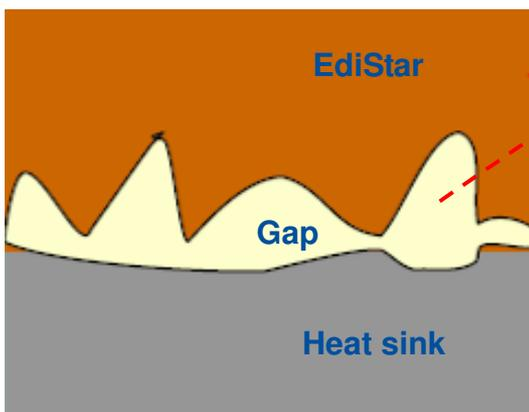
Without the applied force on Edistar, the gap between Edistar and heat sink will be filled with air. The thermal path would be affected such that the thermal resistance between the medium will increase.
