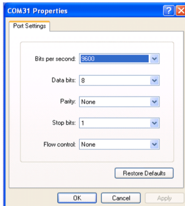
Figure 5. 9600 bps With No Flow Control
