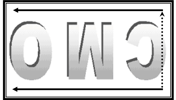
RPF = high: display with 180degree rotation
