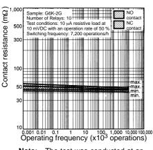
Note: The test was conducted at an ambient temperature of 23°C.
