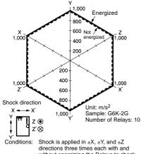
directions three times each with and without energizing the Relays to check the number of contact malfunctions.
