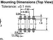
Mounting Dimensions (Top View) Tolerance: ±0.1 mm
