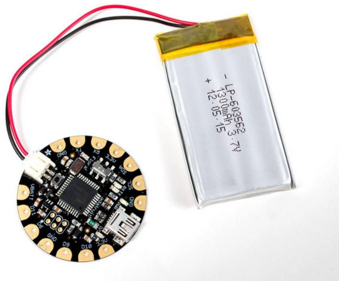
More advanced users may wish to use a rechargeable [lithium polymer battery \(http://adafru.it/258\)](http://adafru.it/258) for their smaller size and longer duration. These batteries pose added risk if abused, shorted, bent, crushed, or punctured. FLORA does not have onboard charging, so you would also need a separate [LiPoly charger \(http://adafru.it/259\)](http://adafru.it/259).
