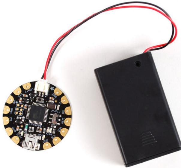
After loading your program onto the FLORA, you'll want to unplug the USB cable and go portable with battery power! USB will always power the board, but battery power (through the JST connector) can be turned on and off with Flora's onboard switch (near the "Flora!" text on the board). We recommend our [3xAAA holder \(http://adafru.it/727\)](http://adafru.it/727) for beginners, which conveniently plugs into FLORA's JST port.
