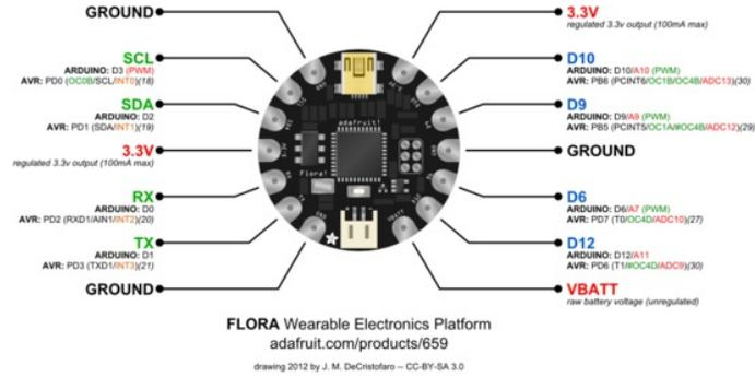
For handy reference, we've created this pinout diagram illustrating all the alternate functions for each of the pins on the FLORA.
