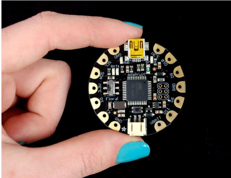
FLORA is Adafruit's wearable electronics platform. We designed it from the ground up to provide the best experience for Adafruit's community of makers, hackers, crafters, artists, designers and engineers. It's built around the Atmega32u4 chip, which has built-in USB support. No pesky special cables or extra parts for programming, just plug it in and get started making the wearables project of your dreams! Works on Windows and Mac.
