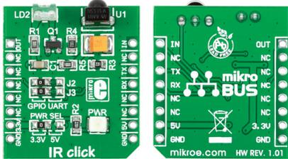
IR Click™ is an add-on board in mikroBUS™ form factor. It's a compact and easy solution for adding infrared (IR) module to your design. It features **TSOP38338** IR receiver module as well as **QEE113** IR emitting diode. IR Click™ communicates with the target board microcontroller via **mikroBUS™** UART (Tx, Rx), AN, and PWM lines. The board is designed to use 3.3V and 5V power supply. LED diode (GREEN) indicates the presence of power supply.
