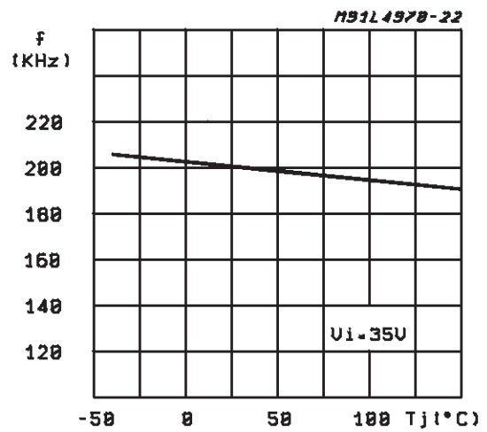
Figure 17: Switching Frequency vs. Junction Temperature (see fig 5)
