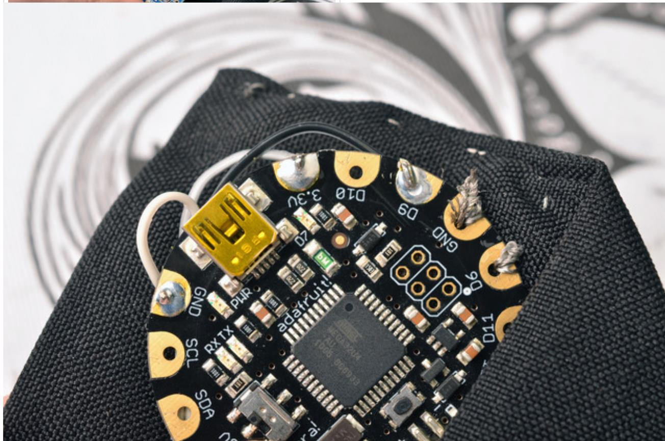
Back at the Flora end of the board, solder the corresponding wires to 3.3V, GND, and D9.
