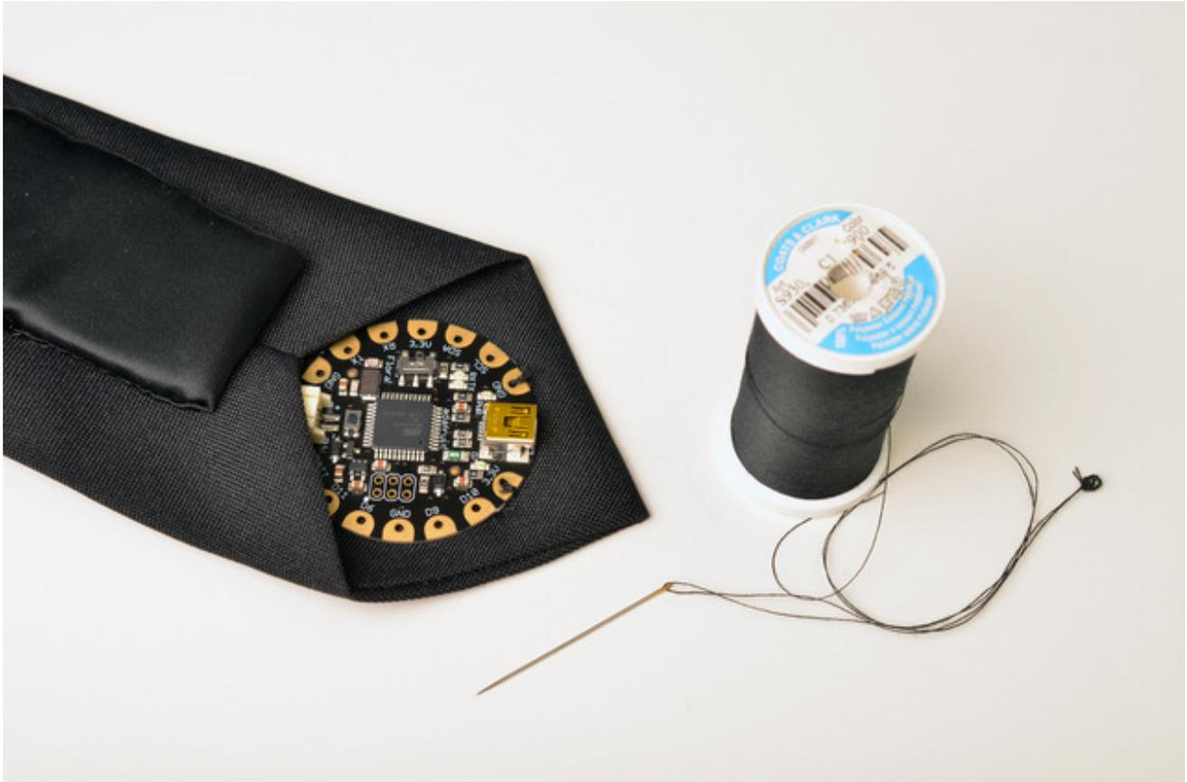
Tack your Flora in place with plain thread by stitching some unused pads to the tie. Try to just stitch to the back surface of the tie so the front fabric remains smooth.
