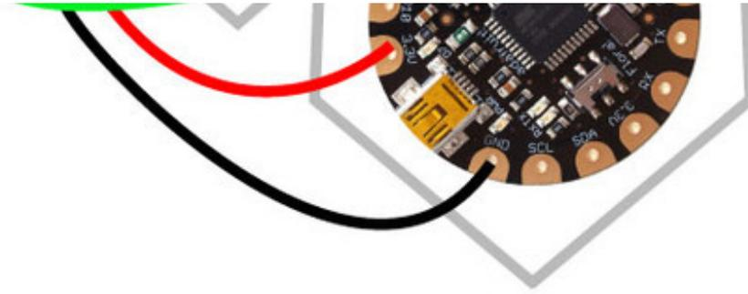
The Flora pixels are all connected to common ground bus, as well as a common power bus connected to VBATT. The Flora pixel data bus is connected to D6. The microphone amplifier is connected to 3.3V, GND, and D9.
