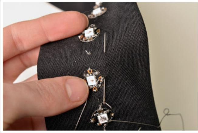
Once you've stitched a few pixels, test for shorts with your multimeter (make sure your long power and ground threads aren't touching), and fire up the NeoPixel library test code to ensure your fledgeling circuit is all good so far.
