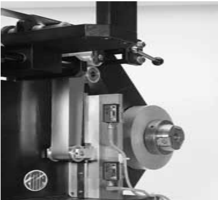
▲ The WT 160 miniature photoelectric proximity switch is used in film processing and for controlling belt tension.
