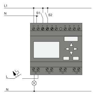
S1 switches input I1, while S2 switches input I2. The load is connected to the relay Q1.
