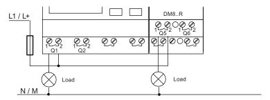
Protection with automatic circuit-breaker, max. 16 A, characteristics B16, e. g.: Power circuit-breaker 5SX2 116-6 (if required)
