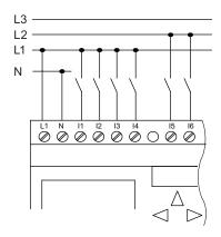
The inputs of these devices are arranged in 2 groups, each consisting of 4 inputs. Different phases are only possible between blocks, but not within the blocks.
