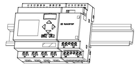
Repeat the digital module steps to mount further expansion modules.
