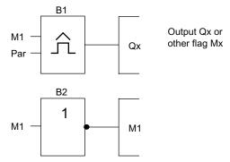
2. Configure the threshold trigger as shown below. A pulse is generated in each program cycle due to the inverted flag. The trigger interval is set to 2 seconds.
