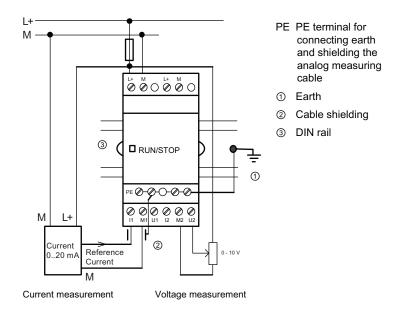
The illustration above shows an example of four-wire current measurement and two-wire voltage measurement.
