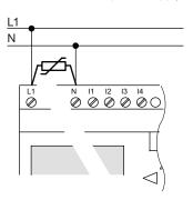
To suppress surge voltages, install varistors (MOV) with an operating voltage at least 20 % above the rated voltage.
