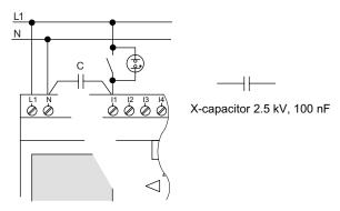
Take into account the quiescent current of any 2-wire proximity switches used. The level of the quiescent current of some 2-wire proximity switches is high enough to trigger a logical "1" signal at the LOGO! input. You should therefore compare the quiescent current of the proximity switches with the technical data of inputs (Page 241).
