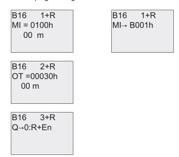
MI is the configurable time interval. The permissible range of values is 0 to 9999 hours.
