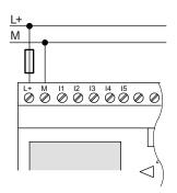
Protection with safety fuse if required (recommended) for:
