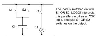
Translated into a LOGO! circuit program this means: Relay K1 is (at output Q1) is controlled by means of an OR block.
