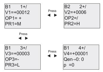
Use the  $\triangleleft$  and  $\triangleright$  keys to navigate between the operand value, operator, and operation priority. To change a value, use the  $\blacktriangle$  and  $\blacktriangledown$  keys to scroll through value choices for each value. Use the  $\triangleleft$  key to navigate from one screen to the previous screen when the cursor is on the V1..V4 line, and the  $\triangleright$  key to navigate to the next screen from the PR1..PR3 line. Use the OK key to accept changes.
