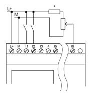
The inputs of these devices are not isolated and therefore require a common reference potential (chassis ground ).
