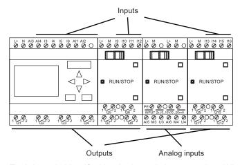
Each input is identified by the letter I plus a number. When you look at LOGO! from the front, you can see the input terminals at the top. Only analog modules LOGO! AM 2 and AM 2 PT100 have the inputs at the bottom.
