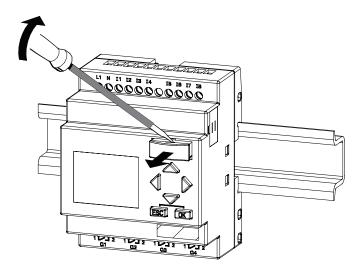
To remove a battery card, or combined memory/battery card, slide a screwdriver into the slot on the upper surface of the card until it engages in the back, then with the screwdriver engaged, pull the card out with your hand.
