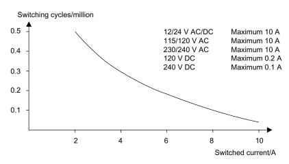
Switching capacity and service life of the contacts with high inductive load to IEC 947-5-1 DC 13/AC 15 (contactors, solenoid coils, motors):
