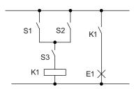
Load E1 is switched on and off by means of the switches (S1 OR S2) AND S3.
