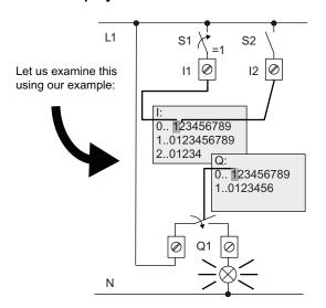
When switch S1 is closed, the status at input I1 is high.
