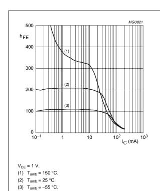
Fig.2 DC current gain; typical values.
