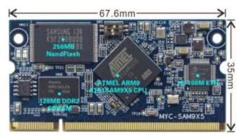
Figure 1-8 MYC-SAM9X5 CPU Module Top-view
