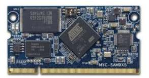
Figure 1-4 MYC-SAM9X5 CPU Module Controller Board of MYD-SAM9X5
