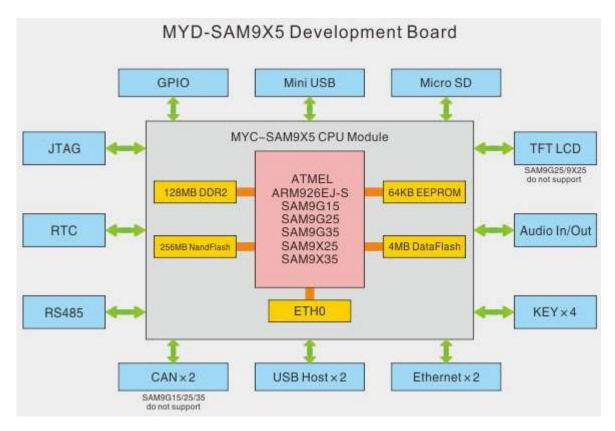
Figure 1-5 Function Block Diagram of MYD-SAM9X5
