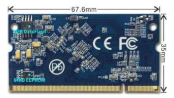
Figure 1-9 MYC-SAM9X5 CPU Module Bottom-view
