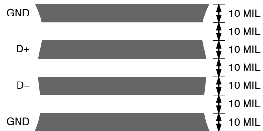
Figure 17. Arrangement of Signal Tracks
