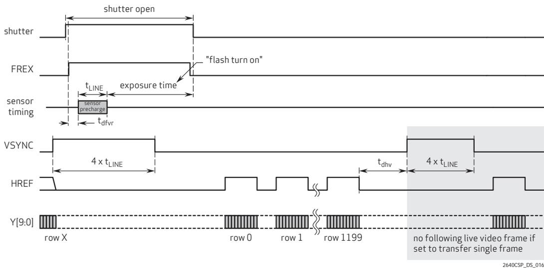
**Figure 17 Frame Exposure Mode Timing with EXPST\_B Asserted**
