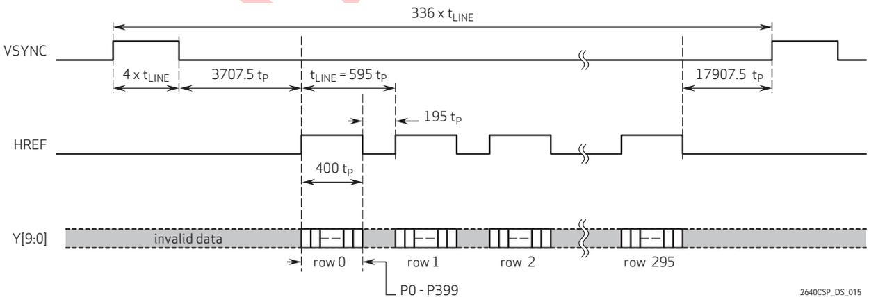
**Figure 16 Frame Exposure Mode Timing with EXPST\_B Staying Low**
