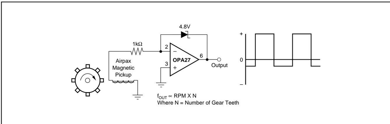
FIGURE 21. Magnetic Tachometer.
