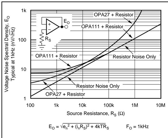
FIGURE 5. Voltage Noise Spectral Density Versus Source Resistance.
