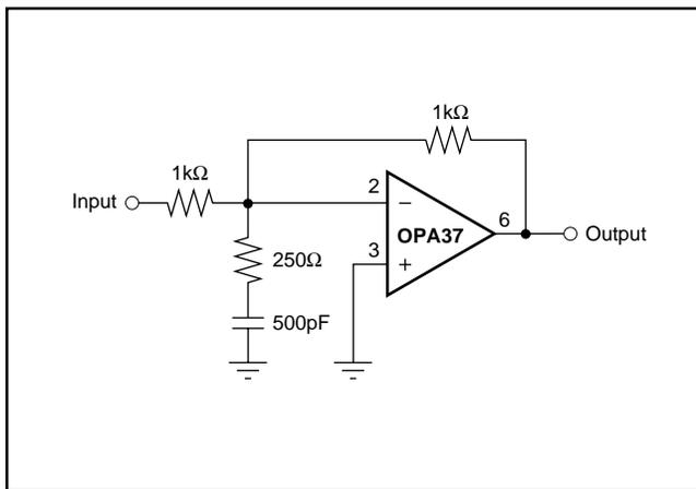
FIGURE 9. High Slew Rate Unity-Gain Inverting Amplifier.
