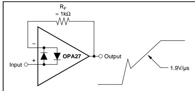
FIGURE 6. Pulsed Operation.
