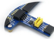
Connecting to EEPROM Board
