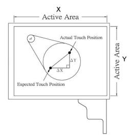
This test is to calculate the difference between the actual touch position and the expected touch position, which
