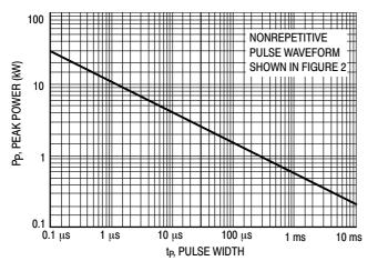
Figure 1. Pulse Rating Curve
