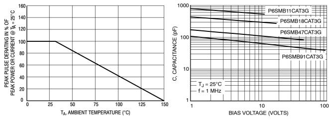
Figure 3. Pulse Derating Curve
