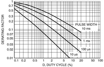
Figure 7. Typical Derating Factor for Duty Cycle
