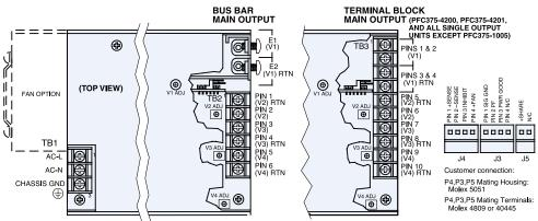
INPUT & OUTPUT CONNECTIONS: 6-32 SCREW TERMINAL ON 0.375" (9.5mm) CENTERS
