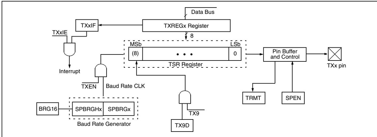
**FIGURE 20-4: ASYNCHRONOUS TRANSMISSION**
