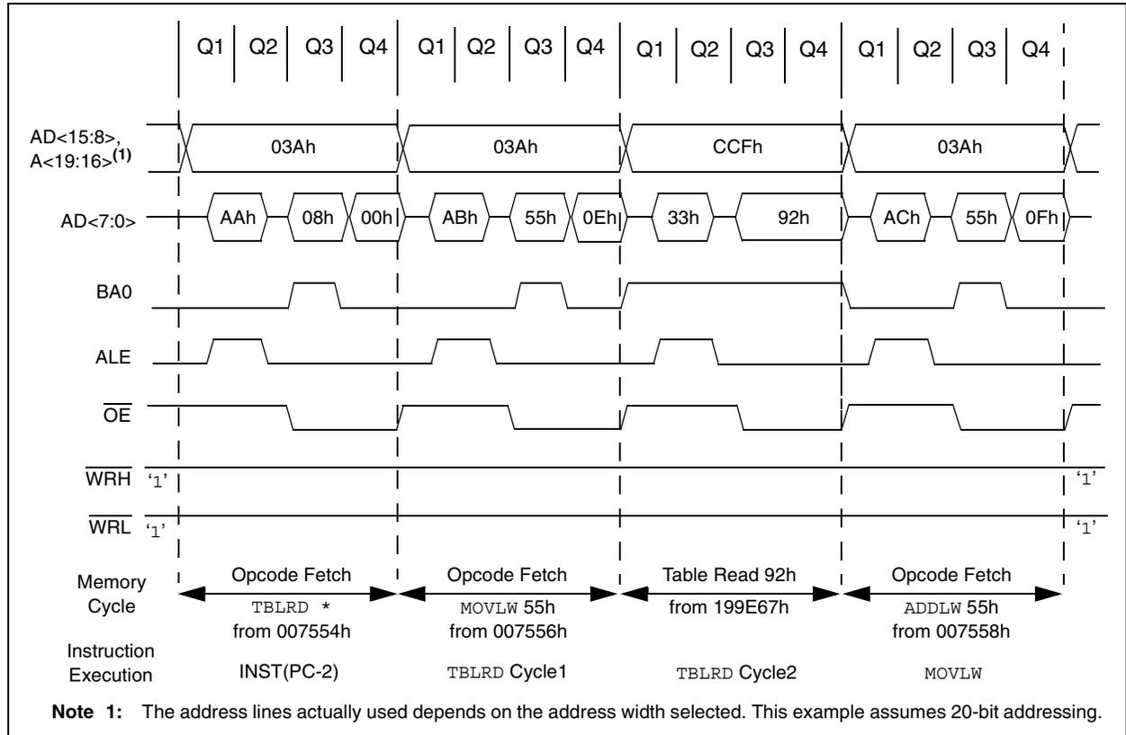
**FIGURE 7-9: EXTERNAL BUS TIMING FOR TBLRD (EXTENDED MICROCONTROLLER MODE)**
