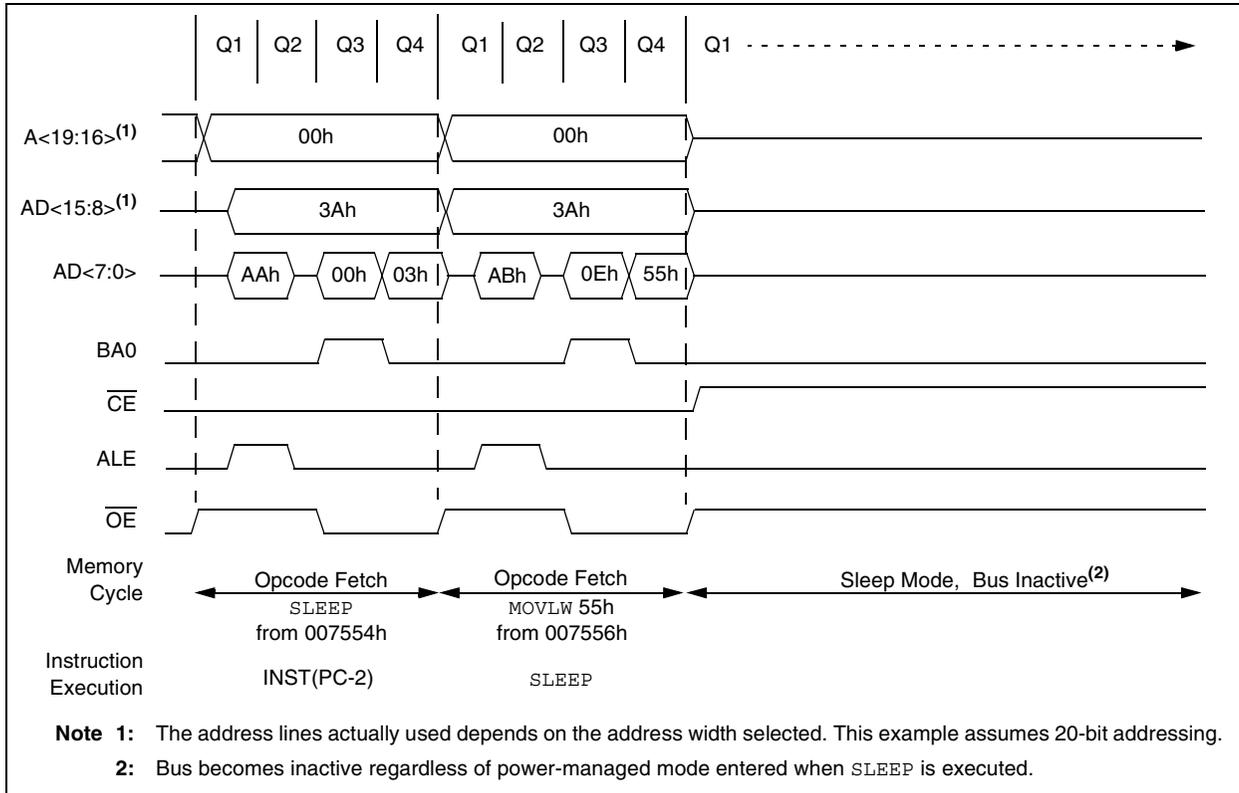
**FIGURE 7-11: TYPICAL OPCODE FETCH, 8-BIT MODE**
