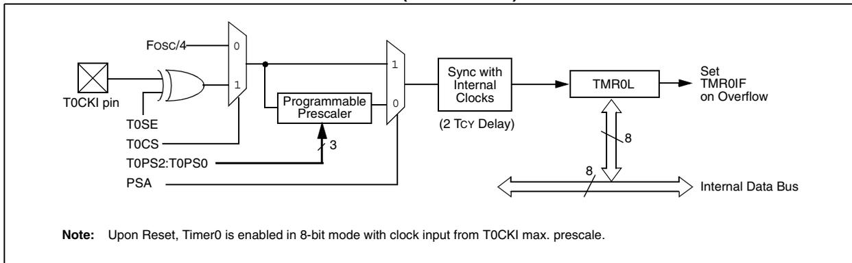
**FIGURE 12-2: TIMER0 BLOCK DIAGRAM (16-BIT MODE)**
