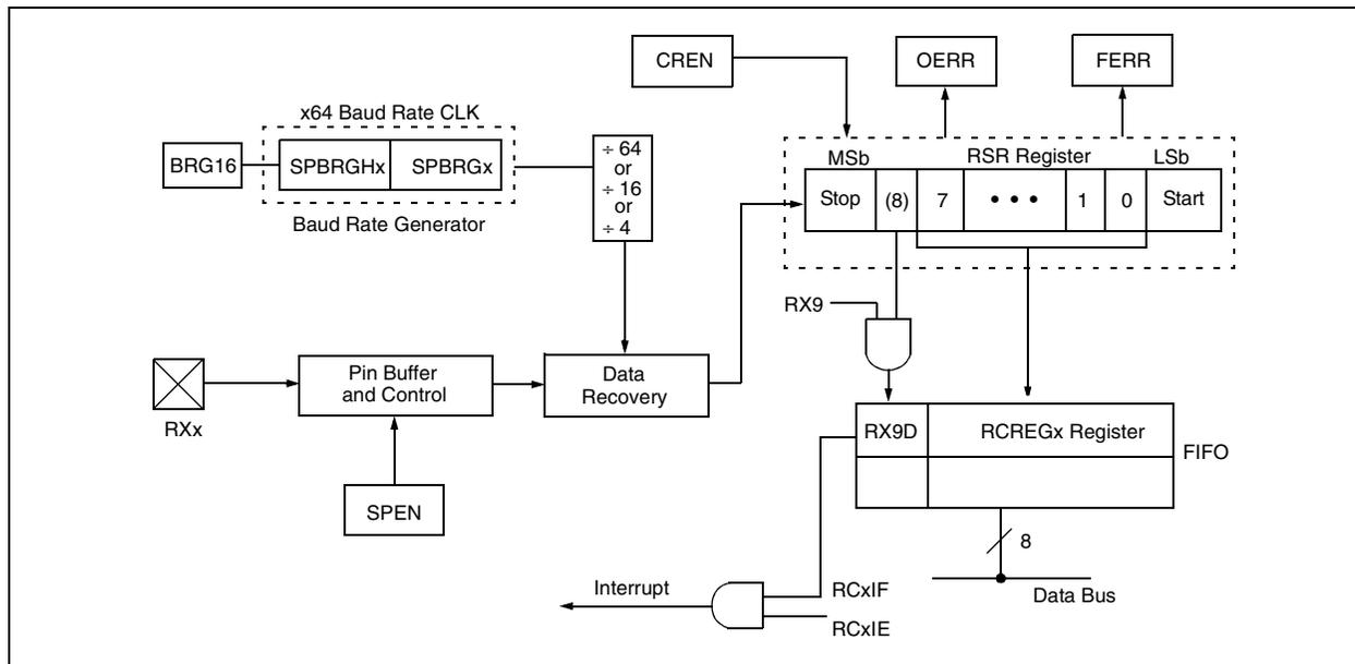
**FIGURE 20-7: ASYNCHRONOUS RECEPTION**
