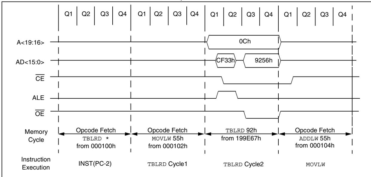
**FIGURE 7-6: EXTERNAL BUS TIMING FOR SLEEP (MICROPROCESSOR MODE)**
