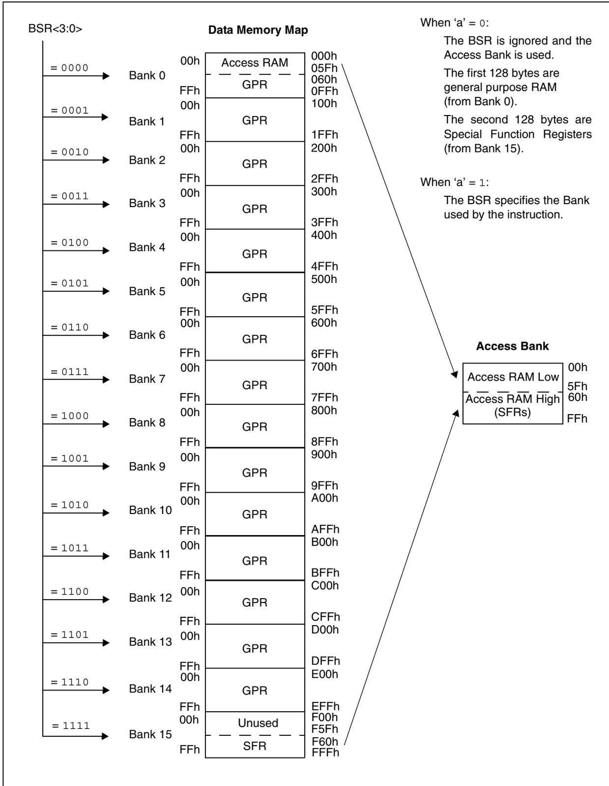
**FIGURE 5-7: USE OF THE BANK SELECT REGISTER (DIRECT ADDRESSING)**
