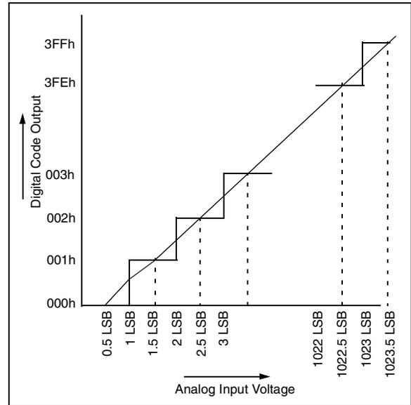
**FIGURE 21-3: ANALOG INPUT MODEL**
