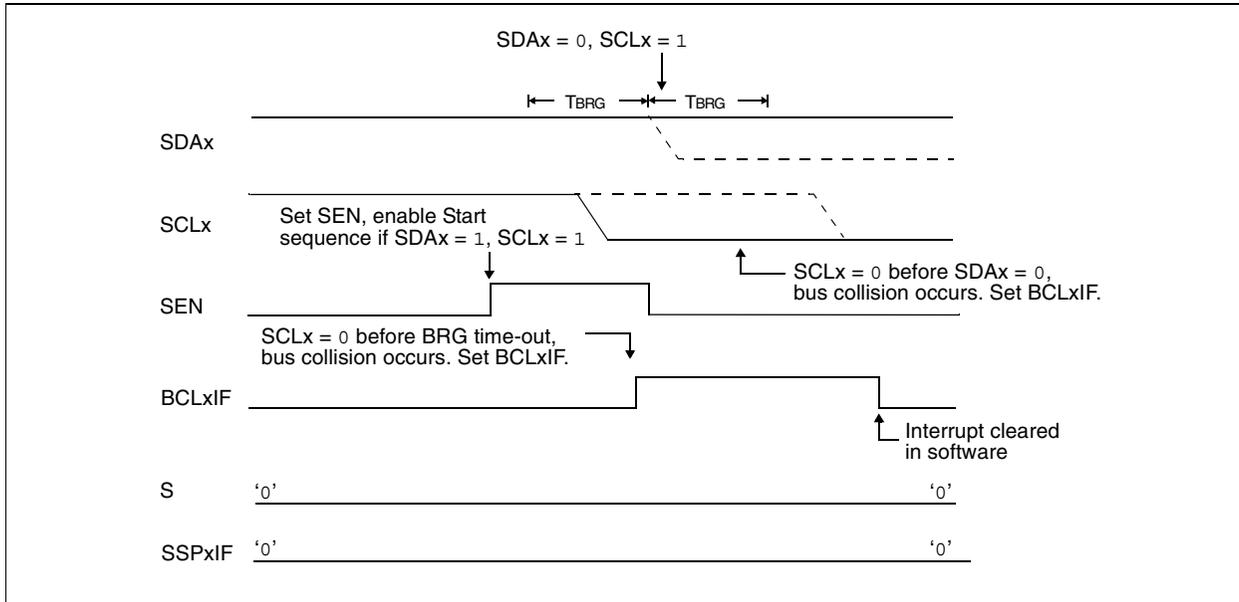
**FIGURE 19-28: BRG RESET DUE TO SDA ARBITRATION DURING START CONDITION**
