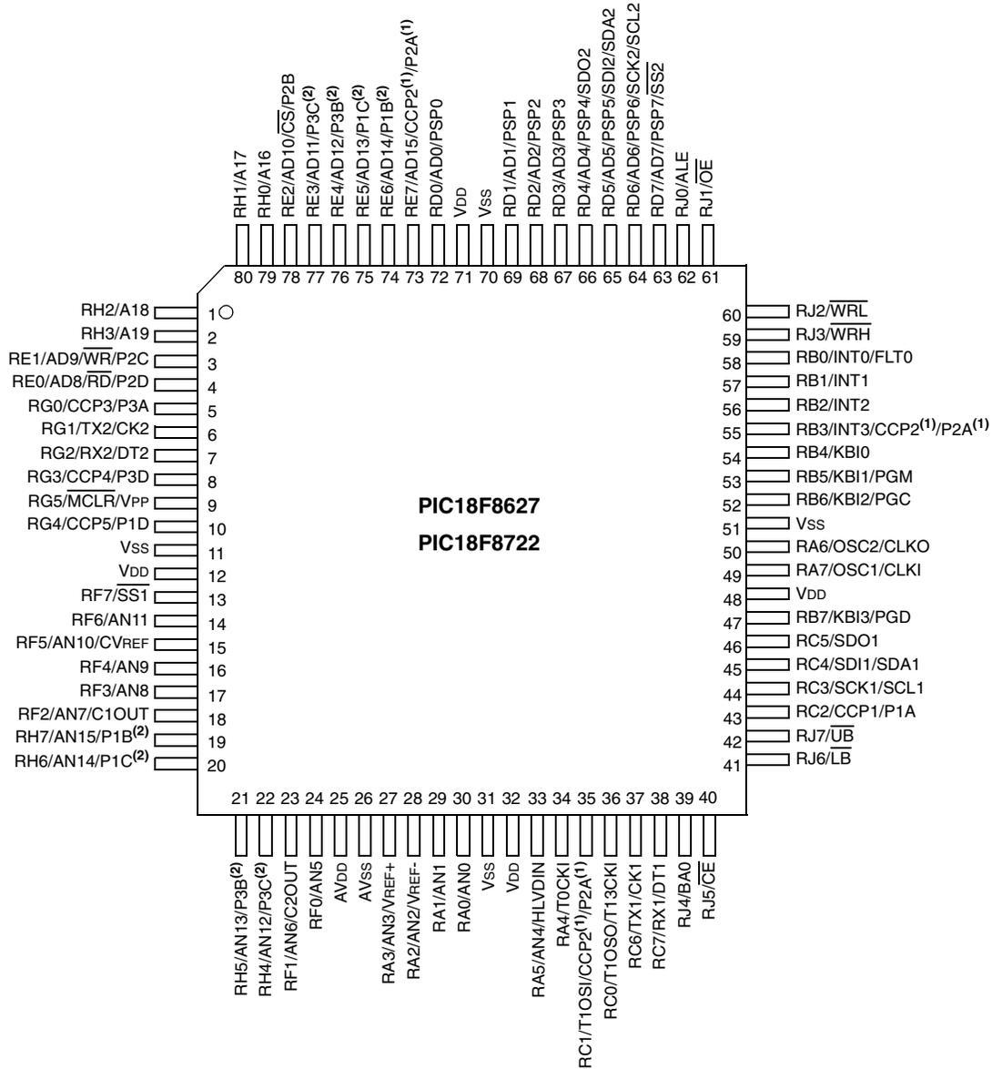
**Note 1:** The CCP2/P2A pin placement is determined by the CCP2MX configuration bit and Processor mode settings.
