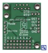
All of the ports are conveniently labeled on the back of the PCB. This servo controller can be reset directly from a serial port using the DTR or RTS handshaking lines. Other unique features include individual servo speed and range control. Three diagnostic LEDs get you up and running quickly.
