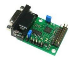
The Pololu serial 8-servo controller allows you to control up to eight RC servos with almost any robot controller or computer. Connect multiple units to the same serial line to control up to 128 servos independently.
