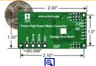
Simple High-Power Motor Controller 18v25 or 24v23 bottom view with dimensions.
