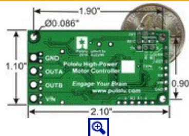
Simple High-Power Motor Controller 18v15 or 24v12 bottom view with dimensions.
