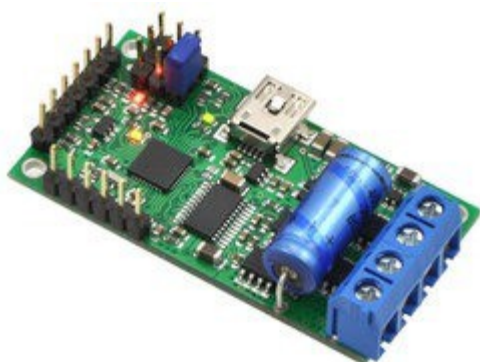
Simple High-Power Motor Controller 18v15 or 24v12, fully assembled.
