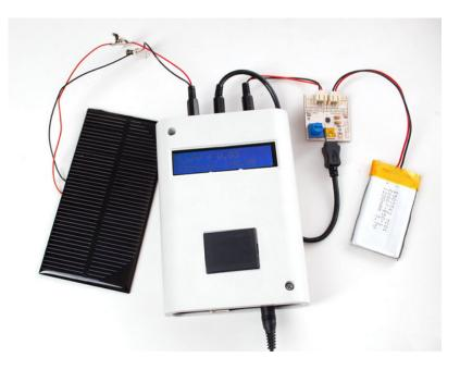
This design is intended for  $\sim$ 6V panels, single Lithium Polymer cells and chargers. It can very easily be adapted to any kind of panel and charger, you'll just need to adjust the resistor dividers and such!
