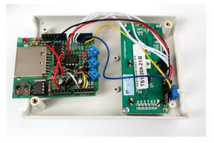
Then try out the LCD by uploading the sketch (http://adafru.it/c8t). You should get the LCD working even if it's not displaying anything.
