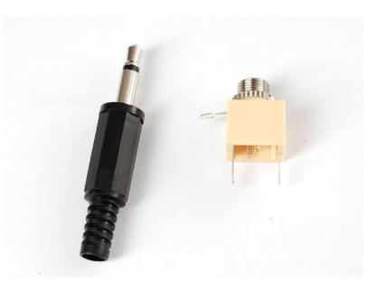
Start with the JST cable that goes to the charger output (to measure the lipo). Unscrew the plug, slip thru the wire, Then solder each pin to crimpies. As a rule, you should always make 'sleeve' or 'ring' ground and 'tip' positive signal. Keeps things easy to track!
