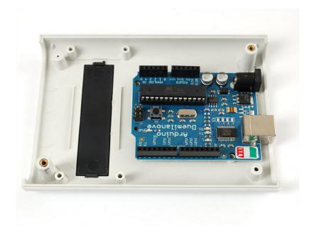
Attach! Use two screws, the third won't fit because the Arduino drill is too small.
