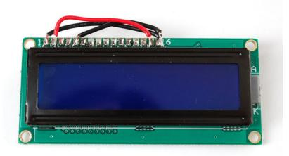
And get rid of that pin as well as pins #1 and #2 (they are close to the mounting post so we'll connect to pins #15 and #16 instead).
