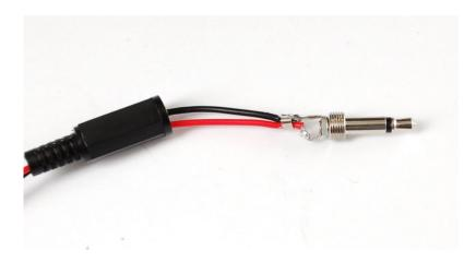
Next, the miniB usb cable is stripped and the red and black wires pulled out (http://adafru.it/c8u). We also use some heatshrink to protect the end of the cable.
