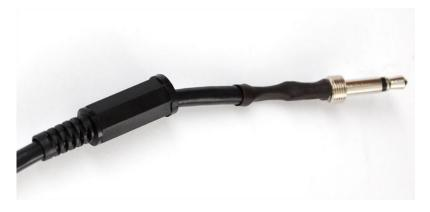
Next, the jacks. Connect any stranded wire to the sleeve and tip connections as shown.
