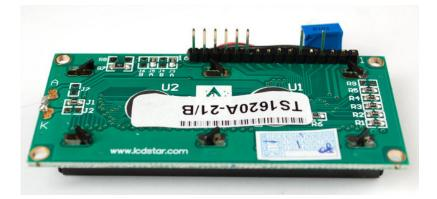
Now we have the used 8 pins, from left to right: ground, power, D7 thru D3, RS and EN. Connect sockets.
