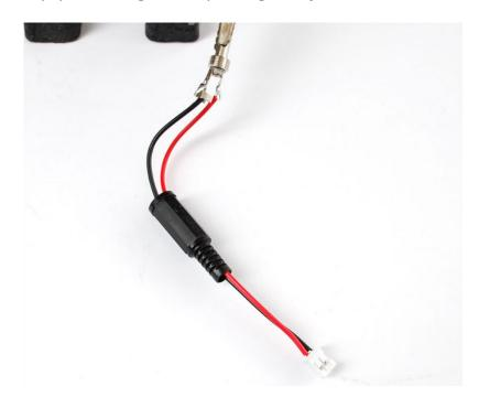
Crimp, making sure not to short the wires. This can be a bit challenging so use a multimeter to test!
