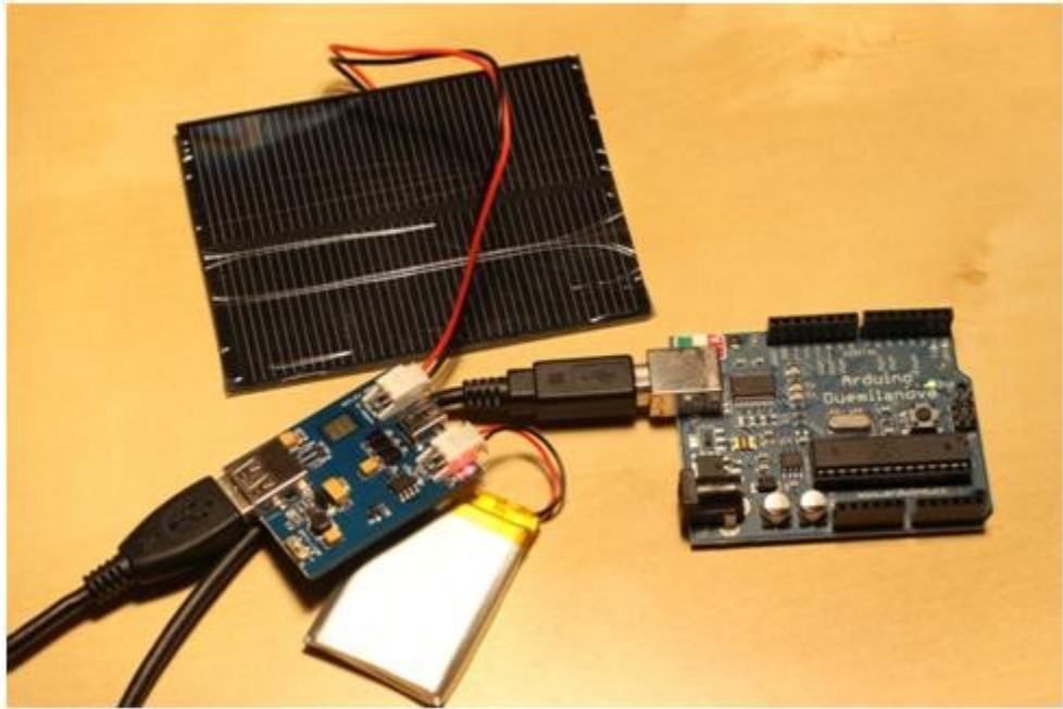
Lipo Rider powering an Arduino Duemilanove (not strict an outdoor sensor in this case as I have not connected any sensor and it is not outdoor, but you get the point )
