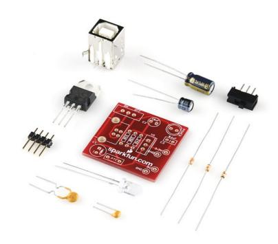
**Description:** A very simple breadboard power supply kit that takes power from any USB port and outputs a fuse protected and regulated 3.3V. The .1" headers are mounted on the bottom of the PCB for simple insertion into a breadboard. Pins labeled 5V/GND 3.3V/GND plug directly into the power lines. When you plug this board into a breadboard you must be aware that the unused power and ground pins will
