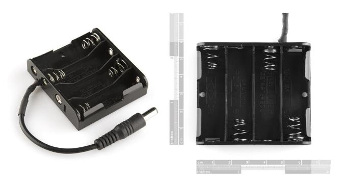
**Description:** This is a simple 4 cell AA battery holder. The 5 inch cable is terminated with a standard 5.5x2.1mm, center positive barrel jack connector.
