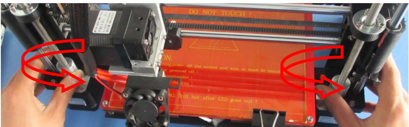
if the distance is too small, we could twist the 2 couplings clockwise simultaneously a little bit, until the distance reach to the reference,
