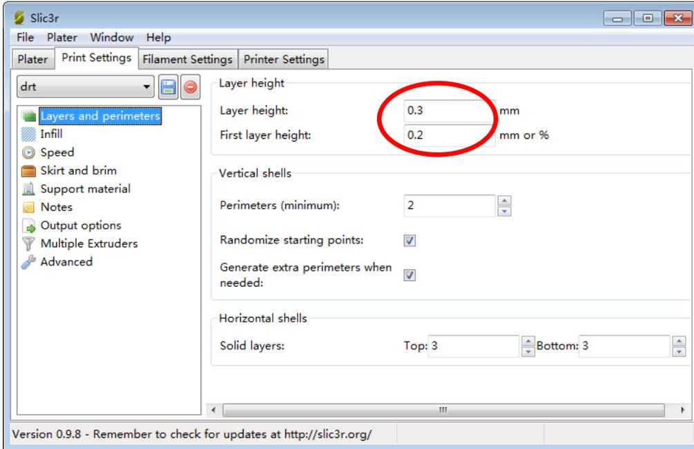
Layer height is suggested 0.3mm, first layer height 0.2mm
