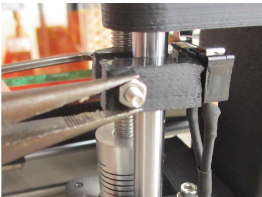
After adjust one corner, don't forget to adjust the other 3 corners, during adjust the other 3 corners, there is no need to adjust the Z end-stop, we could set the screws on the heat bed, if the distance is too large, use the needle-nose pliers the fix the nut,, use M2.5 hex key to loosen the screw counterclockwise as the below picture, when you are doing that, check the distance, reach to the suggested distance is OK
