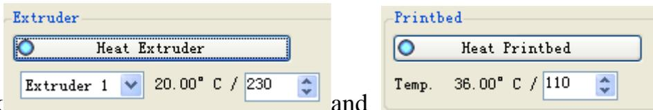
Click  and , the temperature will rise up. When the extruder temperature rise to 230(If PLA, the temperature could be 190), click  , check whether the filament is extruded fluently. Refer to the below picture:
