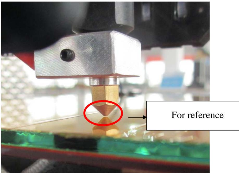
If the distance of the four corners is almost the same as reference, and there is not big difference, we don't need to adjust the machine.
