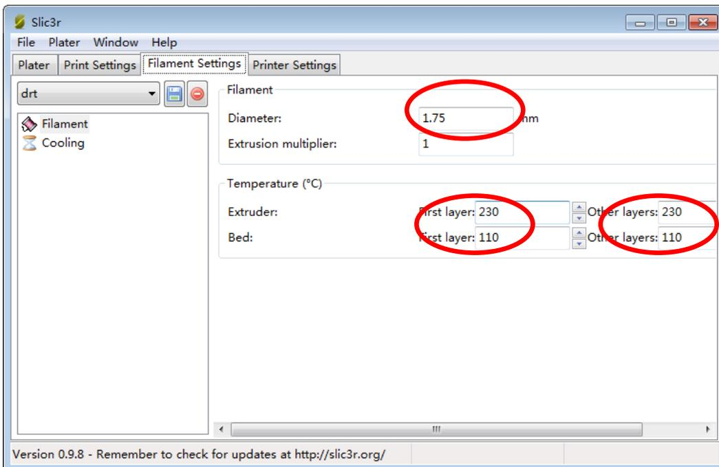
Filament diameter 1.75, extrusion multiplier 1, extruder temperature 230, bed 110(because we are printing ABS)
