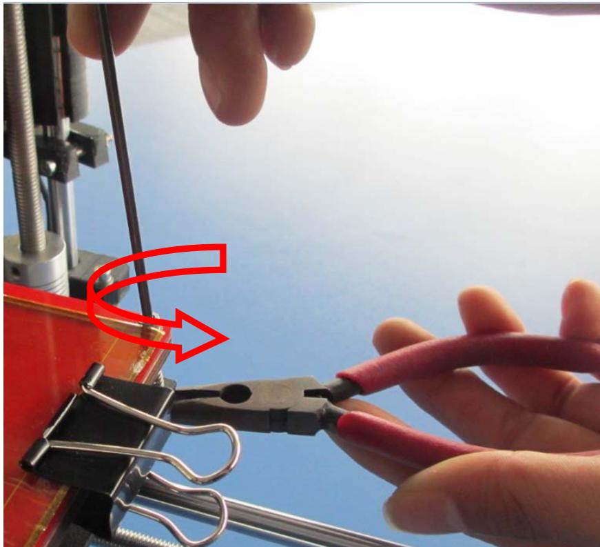
If the distance is too small, we could use the needle-nose pliers the fix the nut, use M2.5 hex key to fix the screw clockwise as the below picture, when you are doing that, check the distance, reach to the suggested distance is OK
