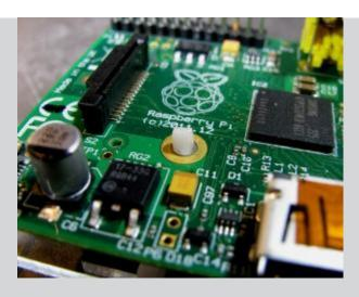
\* \*Note that a few very early model B boards did not have mounting holes on the boards. If you have one of these early boards, you'll need to clip off the loop (it's fairly easy to do with a pair of flush cutters) before continuing.
