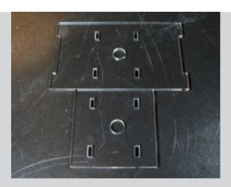
You will notice on the larger of the two panels that the slots are slightly off center. Orientate the panel so that the slots are more towards the left. Stack the larger panel on top of the smaller panel and line the hole and slots up. Now take the PCB mounting clip and snap it into the leftmost pair of slots with the PCB mounting nub closest to you. Snap the other mounting clip in the right pair of slots.
