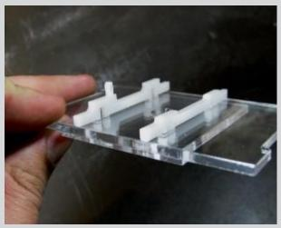
Finally, take the small rectangular piece and orientate its hole with the hole on the bottom piece and place it between the clips. Now insert the brass fitting as shown.
