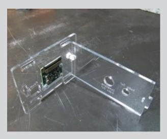
Step 5: Mount the Raspberry Pi on the bottom
