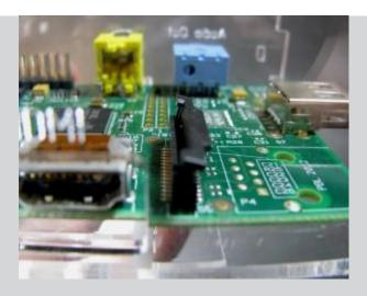
Insert the ribbon cable into the Camera Module connector and lock it in place. Then insert the other end of the ribbon cable into the connector on the Raspberry Pi and lock it in place as well.
