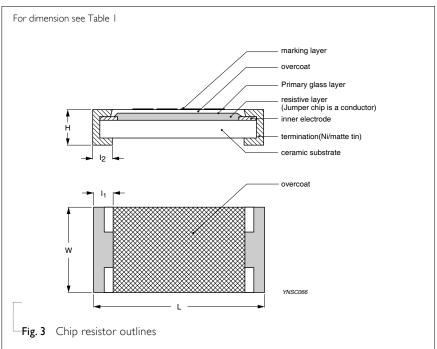
Chip Resistor Surface Mount RC SERIES 0805 (RoHS Compliant)
