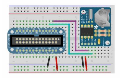
Verify your wiring by running **sudo i2cdetect -y 0** at the command line, you should see ID #68 show up - that's the address of the DS1307! If you have a rev 2 Pi, you will have to run **sudo i2cdetect -y 1** as the I2C bus address changed from 0 to 1
