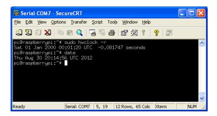
First you'll need to get the right time set on the Pi, the easiest way is to connect it up to Ethernet or Wifi - it will automatically set the time from the network. Once the time is correct (check with the **date** command), run **sudo hwclock -w** to write the system time to the RTC
