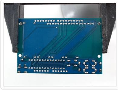
Flip over the PCB and solder in the three legs of the potentiometer and then all 28 pins of the port expander.
