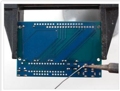
Solder each leg, taking care not to accidentally 'short' two button legs together. The ones for the directional pads are very close!
