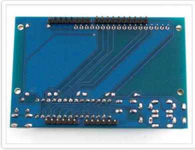
Flip over the shield and place it flat on the table so the long leads of the header stick out.
