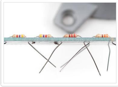
Make sure the resistors all sit nice and flat against the PCB.
