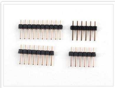
Take a stick of 36 pin header and break off a 10 pin piece, an 8 pin piece and two 6 pin pieces.
