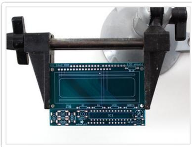
Put the printed circuit board into a vise or board holder, heat up your soldering iron and make sure you're ready to go!
