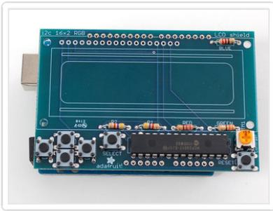
Place the shield right on top. It should fit perfectly where all the short ends of the header fit into the holes of the shield.
