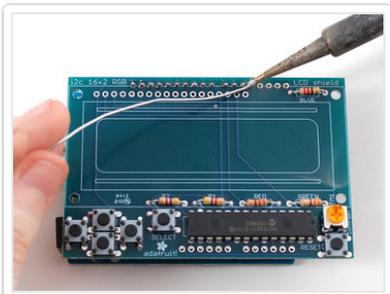
Solder all of the header pins. Even though they aren't used for passing signals, they will make the mechanical connection to the Arduino strong.
