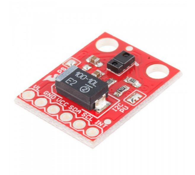
The APDS-9960 RGB and Gesture Sensor board breaks out the pins on the Avago APDS-9960 so you can easily use it in a variety of projects. The APDS-9960 uses the I<sup>2</sup>C interface for communications.
