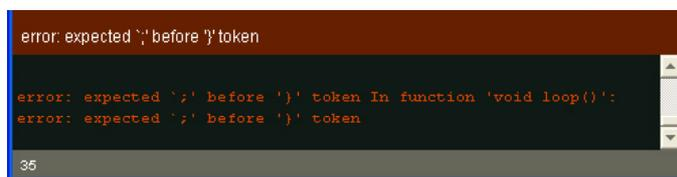
Back to edit the code to fix any error and re-compile again until completely. The Message area shows Done compiling message following the picture below.
