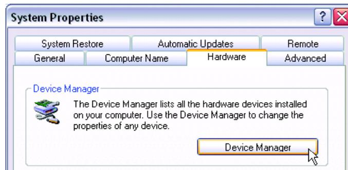
(3) See the list of USB serial port and remember the COM port address to work with ZX-U2S board. Normally it will create COM3 or higher. In this example is COM4
