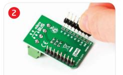
Turn the board upside down, so that bottom side is facing you upwards. Place shorter parts of the header pins in the both soldering pad locations.
