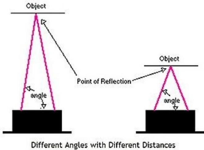
The angles in this triangle vary based on the distance to the object. The receiver portion of these new detectors is actually a precision lens that transmits the reflected light onto various portions of the enclosed linear CCD array based on the angle of the triangle described above. The CCD array can then determine what angle the reflected light came back at and therefore, it can calculate the distance to the object.
