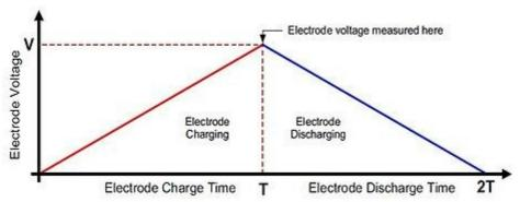
The amount of charge(Q)applied is programmable by setting the charge current(I), And the charge time(T). Once the electrode is charged, the peak voltage(V)at the end of chage is measured by internal 10 bit ADC. This voltage V is reverse proportional to the capatance(C)on the sensing channel.
