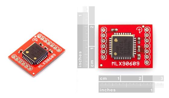
**Description:** This is a simple breakout board for the Melexis gyroscope featuring both analog and digital (SPI) interfaces. Designed for dead reckoning navigation applications, the MLX90609-E2 is a 150 degree/s max rate gyro with low drift and programmable bandwidth, this gyro is perfect for digital stabilization and control.
