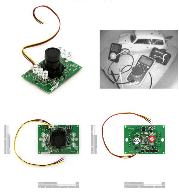
**Description:** This is a high-quality black and white CMOS camera module with high-power infrared LEDs to light up the night. Power the CA-84AC module, hook up any display, monitor, or LCD screen with an RCA input and get vivid black and white video at 500x582 resolution even in completely dark environments. Module is easily mountable and should be powered close to the 12V spec. Comes with high quality optics, all the on board circuitry to output RCA signal, and cable harness.
