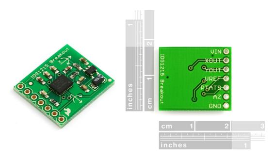
**Description:** This is the breakout board for the IDG1215, which includes an on-board 2.8V regulator and all pins broken out to 0.1" pin holes. The IDG-1215 is an integrated dual-axis angular rate sensor (gyroscope). It uses InvenSense's proprietary and patented MEMS technology with vertically driven, vibrating masses to make a functionally complete, low-cost, dual-axis angular rate sensor. All required
